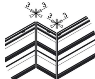
Allow 3mm gap for thermal expansion
