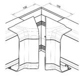
To fit (Internal Bend) mitre trunking base and fit lids allowing 106mm gap from end of trunking to lids, clip covers in place.
