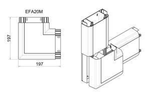
Flat Angle to be assembled as shown in illustration, ensuring that the lids on mating trunking lengths extend beyond base by 35mm to engage with base of fitting and sit 10mm under cover when fitted.
