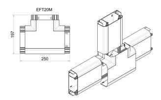
Flat Tee to be assembled as shown in illustration, ensuring that the lids on mating trunking lengths extend beyond base by 35mm to engage with base of fitting and sit 10mm under cover when fitted.
