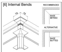
After fixing base to corner, fit covers with offset as shown then clip Internal bend in place.
