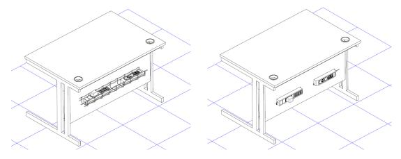
Each unit is fitted with 2 fixing points at either end of the module for ease of mounting and securing the unit in a fixed position. Screw size: No4  $\times$  % Woodscrew should be used - It is recommended not to over tighten the screws or use an impact driver as this may damage the case
