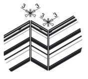
Allow 3mm gap for thermal expansion.
