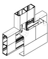
Flat Tee to be assembled as shown in illustration, Fit radius controls before covers, ensure that the lids are recessed enough to allow mouldings to clip to base of the trunking ensuring a good tight fitment.
