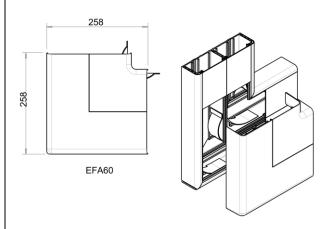
Flat Angle to be assembled as shown in illustration, Fit radius controls before covers, ensure that the lids are recessed enough to allow mouldings to clip to base of the trunking ensuring a good tight fitment
