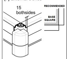
After fixing base to corner, fit radius control than covers with offset as shown then clip External bend in place.
