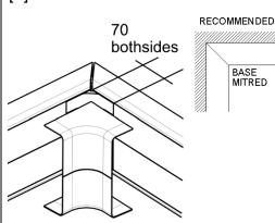
After fixing base to corner, fit radius control then covers with offset as shown then clip Internal bend in place.
