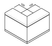
External Bend is supplied as fabrication of base with covers (removable) – fix base to wall and butt up base lengths aligning with LDP1 pins, then fit covers
