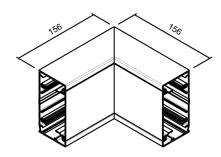
Internal Bend is supplied as fabrication of base with covers (removable) – fix base to wall and butt up base lengths aligning with LDP1 pins, then fit covers
