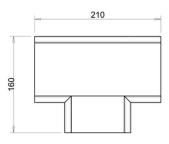
Flat Angles are supplied as fabrication of base with covers (removable) – fix base to wall and butt up base lengths aligning with LDP1 pins, then fit covers
