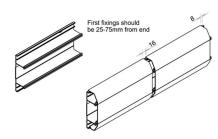
Base to base and Lid to Base bonding on all sections of trunking is recommended to maintain continuity – when fitting fabricated fittings bonding from trunking base to fabrication base is also recommended.
