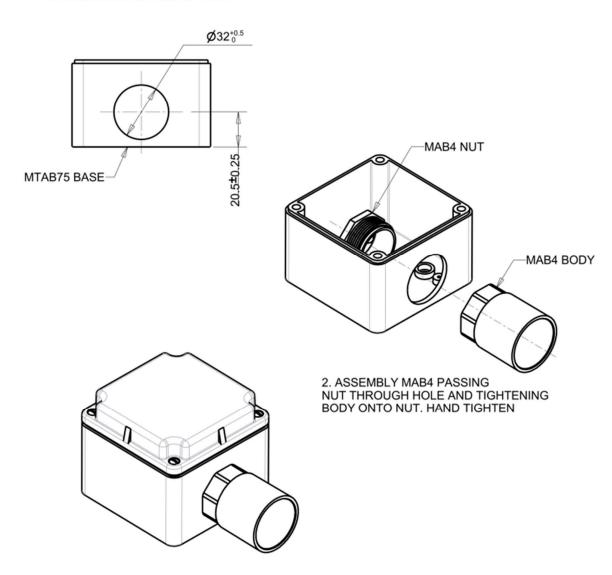
20.5mm height of hole from base is important to reduce any strain on conduit when fixed with saddle straps.
